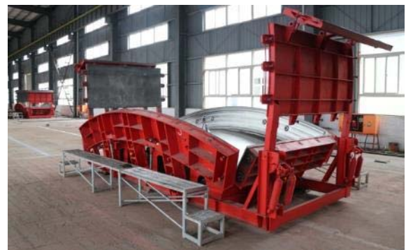
Trail master ring assembly in Dragages Bouygues JV's precast yard (OD13.5m x 2.2m x 0.55m).
