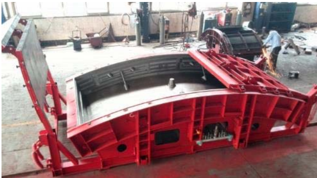
Trail master ring assembly in Dragages Bouygues JV's precast yard (OD13.5m x 2.2m x 0.55m).
